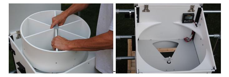
With the Drum removed a sweep and wipe down cleaning can be performed to the cabinet interior. A wash down of the Cabinet interior is not recommended. The Distribution Drum on the other hand can be cleaned and washed down with a garden hose.
